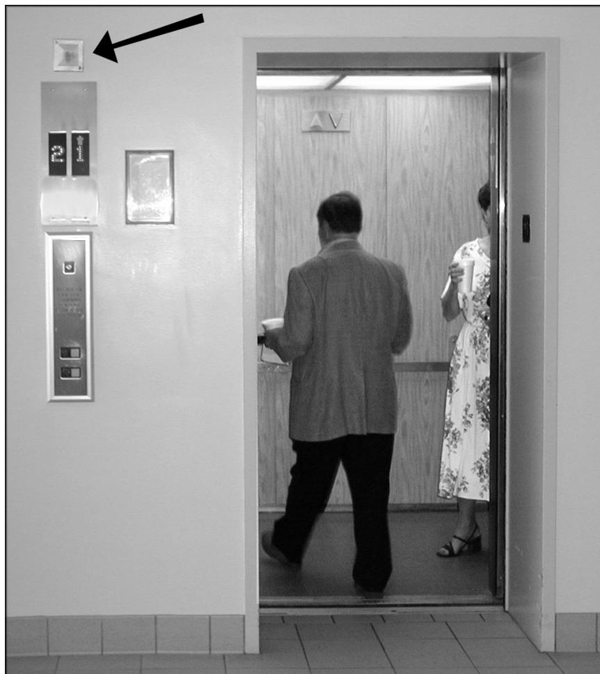
Figure 2.3 shows how the transmitter above a doorway to a building gives an identifying signal whose message names the building. The signal is homed in on to give the user a direct path to the labeled location.
